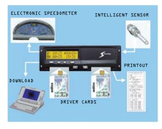
The VU (shown in the centre of the above diagram) has a display, two card slots, a printer, an aperture for connecting download equipment and various control buttons. It holds data on the vehicle's drivers and their periods of driving and duty (when a driver's card has been insterted in the VU), together with data related to faults, attempts to tamper with the system, over-speeding, use of the vehicle without a driver card, calibration details and when data has been accessed.
